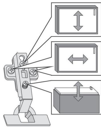
GB Adjusting the doors (adjusting the hinges)
